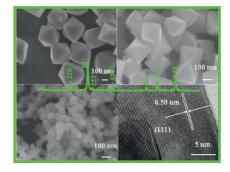
$Fe_3O_4$  octahedra having tunable size, sharp edge length distribution, and uniform shape were prepared by a polyol route. The influence of the dose of  $N_2H_4\cdot H_2O$  on size and shape was investigated.  $Fe_3O_4$  octahedra with edge length in the range 70-1000 nm were synthesized. Interestingly, it is not the edge length but the angles of the octahedra that have the greatest effect on the magnetic properties.
