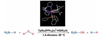
An X-ray crystallographic study showed that the previously reported complexes  $TpRu(PPh_3)(H_a)(\eta^2-H_bSiR_3)$  and  $TpRu(PPh_3)(H_b)(\eta^2-H_aSiR_3)$  should be formulated as  $TpRu(PPh_3)(\eta^3-HSiR_3H)$ , a struc-
