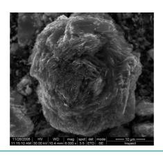
Hierarchically structured  $La_2O_2M@C:Eu^{3+}$  (M = S, Se) microflowers have been successfully prepared by a facile one-pot synthesis at a low temperature of 950 °C by the RAPET technique. The structural (XRD, Raman), morphological (HRSEM, TEM and HRTEM) and optical (UV/Vis) properties of the materials have been studied.
